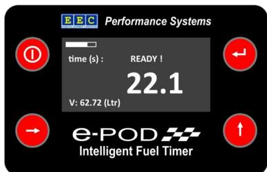
During the fuelling, the high contrast OLED display shows an ascending count in tenths of a second making the operators job child play. When the nozzle is removed from the car, the timer stops instantly and then displays the total time of the process and a calculated volume.
