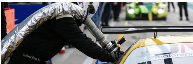
As the Krontec RFC89 does not have any external moving parts for us to trigger the timer from, we took advantage of the Krontec's option to have a proximity sensor on the car side of the coupling.
