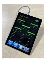
The Wi-POD is normally supplied with a Microsoft Windows tablet PC with software and license preloaded and a USB stick style receiver
