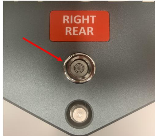
Level each scale to each other scale at the height to suit your application using the built in spirit level.
