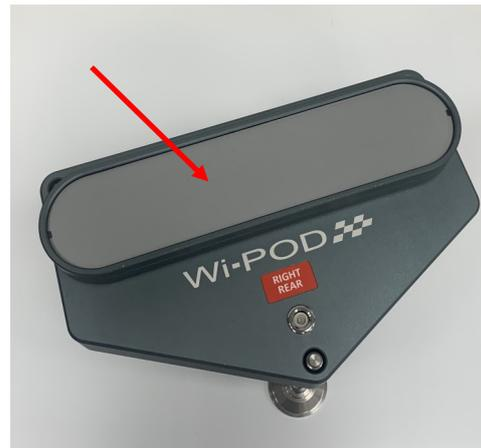
Fit the Wear Plates in position. Do not use without these fitted.
