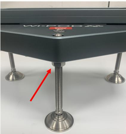
Once they are level, tighten the 3x M12 locknuts on each scale, check level again once tightened and re-adjust if necessary.
