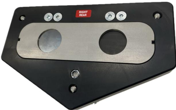
Insert a Load Pad into each hole in the Guide Plate. They are a close fit. If they get stuck, remove and refit very carefully.
