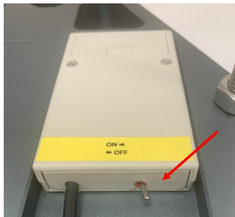
Switch each scale on using the toggle switch on the electrical box underneath. Always switch off when not in use to help battery life,
