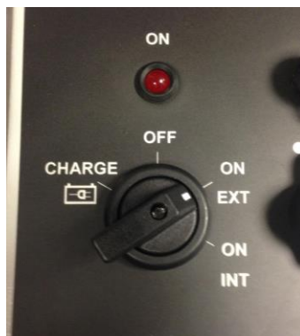
f-POD ON EXTERNAL BATTERY
