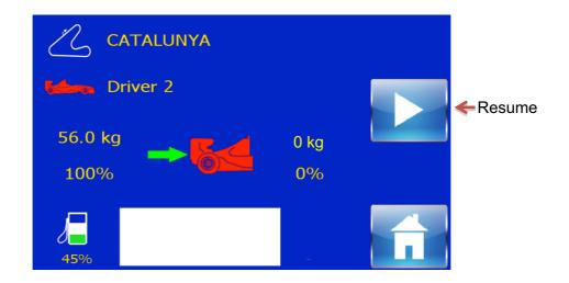
If the E-STOP button is pushed for and reason during fuel transfer, the E-STOP Screen will appear
