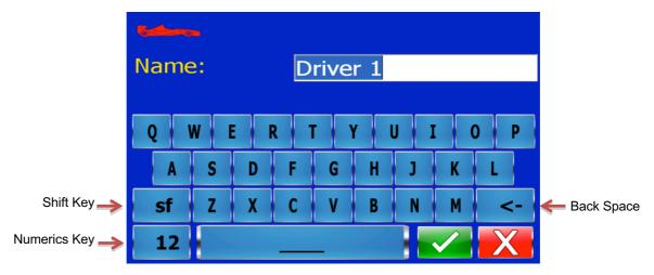
Using the on screen keyboard the operator can edit existing names or add new ones. When the typing is complete, press the green 'Confirm' button to accept. Pressing the red 'Cancel' button returns to the 'User Settings' screen.
