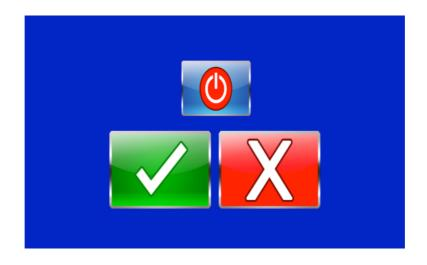
Pressing the green 'Confirm' button will shut down the program. Do not switch off the Control Switch until the touch screen has completely shut down Pressing the red 'Cancel' button will return to the 'Home' screen.
