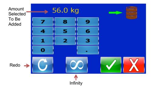
Using the numeric keys, select the required amount to be added, which will be displayed at the top of the screen, then press the green 'Confirm' button to accept.
