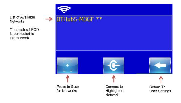
Press SCAN to search for available networks which will show in the list above box To select from list, touch the name of the network required to highlight it then press the CONNECT button. The password screen will open. Type in the password and the green TICK button to accept. \*\* should appear at the end of the network name to show you are connected. Also you should now see the WiFi signal strength meter on the home screen.
