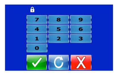
To 'Log In' a numeric PIN code must be entered. Entry to the next stage is automatic. If a mistake is made then pressing the blue 'Redo' button will allow the operator re-enter their code. Default operator PIN code is '1111'.
