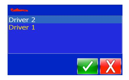
The operator touches the name of the driver/car from the list to highlight, then presses the green 'Confirm' button to select. Pressing the red 'Cancel' button cancels the selection and returns back to the log in screen.
