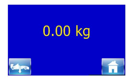
Pressing the NUDGE button will run the pump for a set amount of time to transfer a minimum amount of fuel, which will show on the weight reading. The NUDGE button can be pressed several times to get close to the desired amount. When that is achieved, press the HOME button which will return you to the home screen and record the amount of fuel transferred in the totals report.
