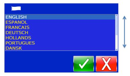
The operator can select an operating language from the list by sliding a finger down the scroll bar, until the required language is displayed. Then by pressing the language type and then pressing the green 'Confirm' button to accept. Pressing the red 'Cancel' button will cancel the selection and return back to the 'User Settings' screen.
