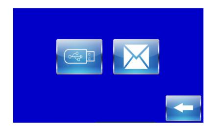
The operator can download the report as a basic CSV format, by inserting a USB memory stick into the socket on the Control Panel, then pressing the 'USB Memory Stick' button.
