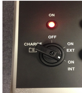
f-POD ON LED INDICATOR ILLUMINATED
